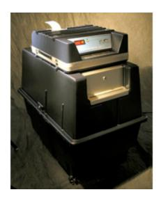
**Brief Description**: As an optical ballot tabulator, the Optech III-P Eagle functions at the precinct level. The Optech III-Eagle consists of an electronic ballot counting device which reads completed ballots by scanning for the voters' marks indicating their voting preferences. The Optech III-Eagle then tabulates the results. When the polls close, the results are both printed on a paper copy and stored to an internal memory card.<sup>1</sup>
